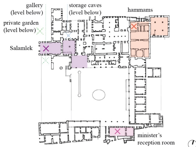
Figure 17: plan of Dar-al-Wousta and datalogger location
